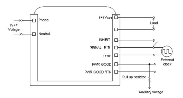
**Note**: PWR GOOD- the load for the pull-up resistor and the auxiliary voltage shown in this diagram should be less than 1mA. The system designer must select the actual values such that no damage can occur to the internal components of the power supply – **consult factory for more information**
