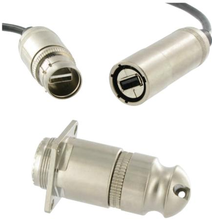
This product offers a new coupling solution, particularly for applications requiring quick disconnect. The system consists of a circular spring within in the receptacle keeping the plug mated, and creating an internal coupling mechanism.
